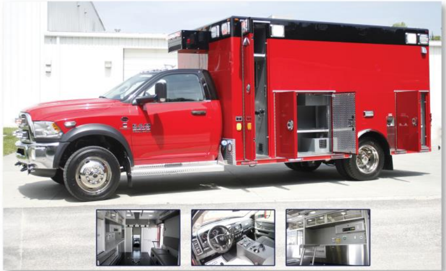
Osage Type 1 mounted on Dodge 4500 chassis, 168" body
