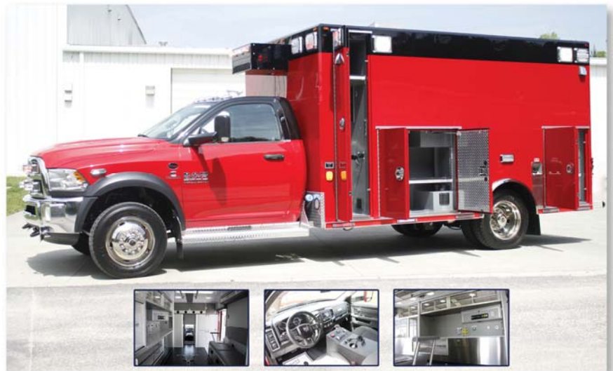
Osage Type 1 mounted on Dodge 4500 chassis, 168" body
